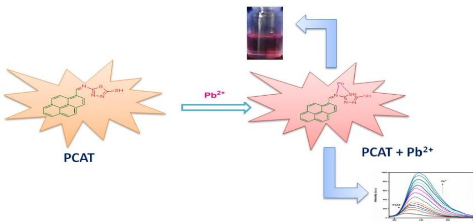
*Graphical diagram for the development of Pb<sup>2+</sup> fluorescence sensor (Chapter -VII)*
