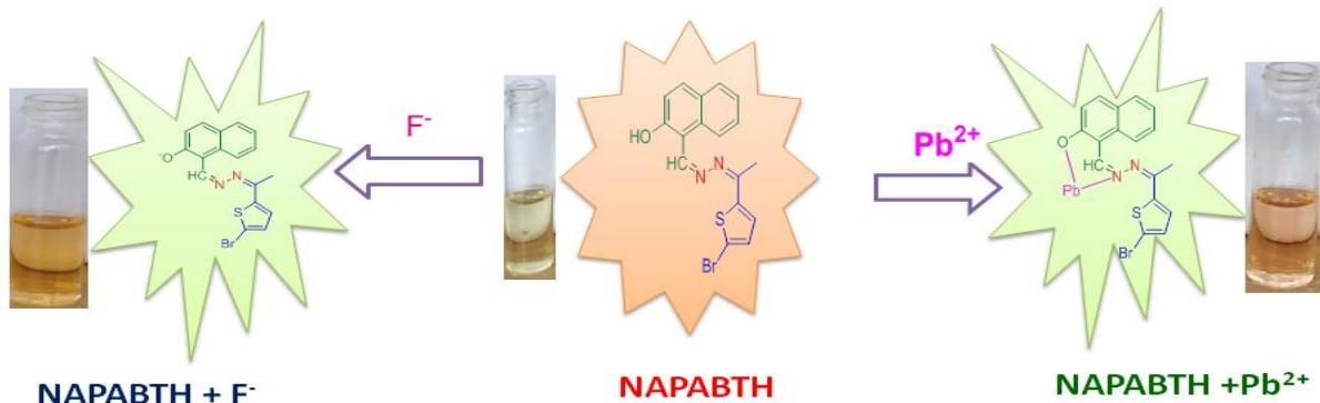
*Pictorial representation of colorimetric sensor for Pb<sup>2+</sup>/F<sup>-</sup> ions by the probe NAPABTH*
