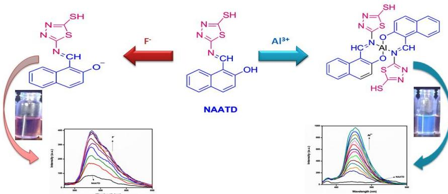
*Graphical diagram for the development of  $\text{Al}^{3+}/\text{F}^-$  ions using NAATD (Chapter -III)*
